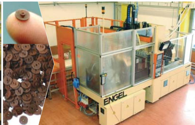
Blum: The Engel machines cover requirements from 250 to 3,000 kN and must meet the highest demands of precision and reproducibility in mass production. A typical example are the tiny disks in TPU (centre photo) which make a vital contribution to the operation and service life of the BLUMOTION system. These sprueless parts are produced on an all-electric ENGEL E-MOTION 80/55 in a 32-cavity mould with full hot runner system and demoulded and sorted by an ENGEL ERC 33/1-EH.
