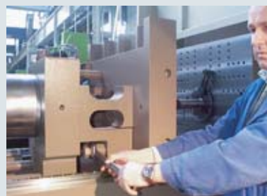
The adjustable, maintenance-free FlexLink not only ensures parallelism of the moving platen during the injection moulding cycle but also transmits the clamping force to the mould.
