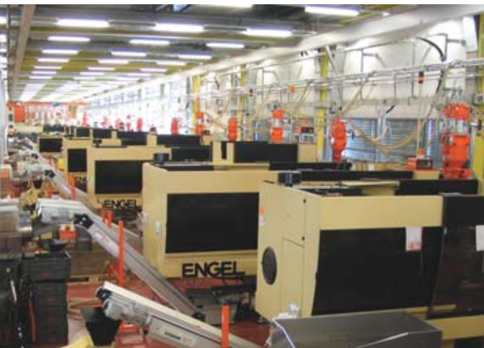
Blum: The Engel machines cover requirements from 250 to 3,000 kN and must meet the highest demands of precision and reproducibility in mass production. A typical example are the tiny disks in TPU (centre photo) which make a vital contribution to the operation and service life of the BLUMOTION system. These sprueless parts are produced on an all-electric ENGEL E-MOTION 80/55 in a 32-cavity mould with full hot runner system and demoulded and sorted by an ENGEL ERC 33/1-EH.
