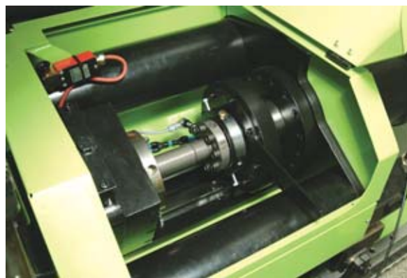
An integrated friction clutch transmits the torque – without stress concentrations – from the drive to the screw.
