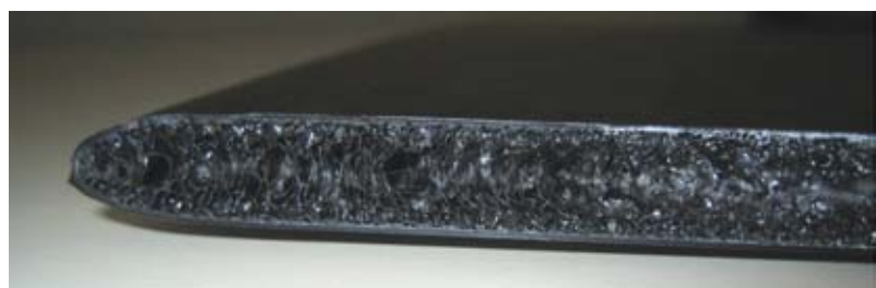
Foamed PP (polypropylene) sheet produced by the MuCell decompression injection moulding process: the initially moulded part (having the appearance of a solid, conventionally moulded part) had a wall thickness of 3 mm. The final thickness of the sheet measures 10 mm.
