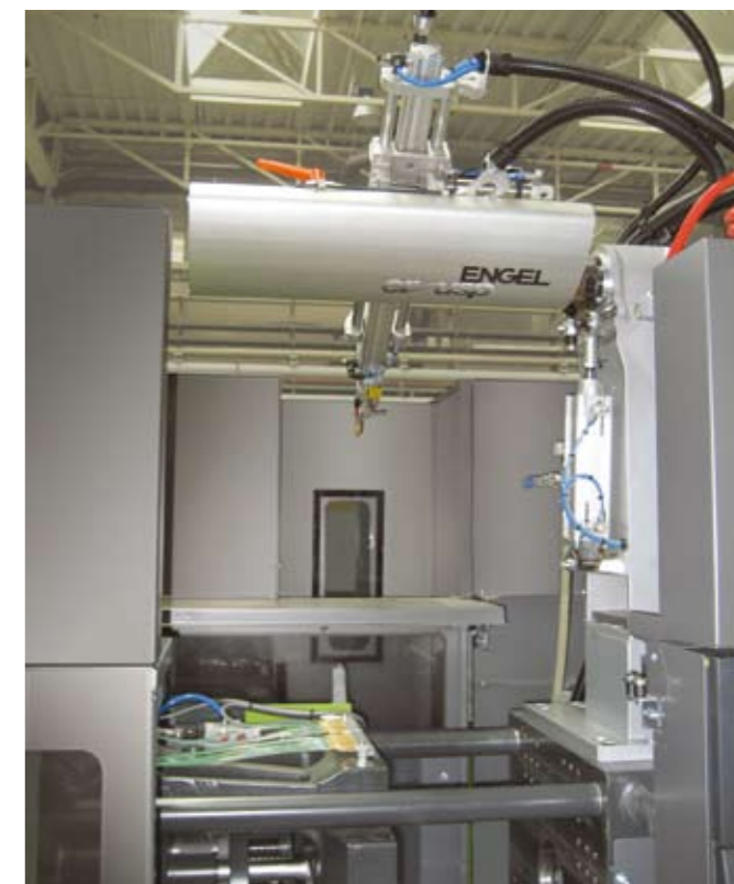
Fast sprue removal and cutting with the tried-and-trusted ENGEL ER-USP automation solution
